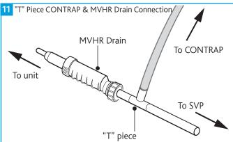
When using a "T" Piece to connect the CONTRAP drainage and the MVHR drain pipework the MVHR drain must always be fitted before the "T" Piece to prevent condensate from feeding back into the MVHR system.
